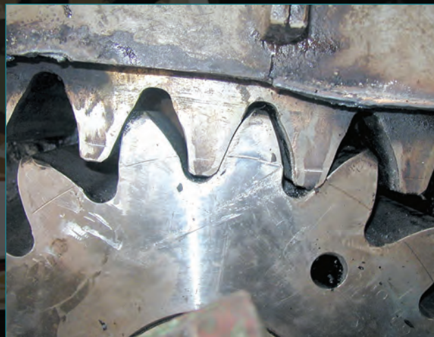
Figure 3. Severe gear profile wear.
