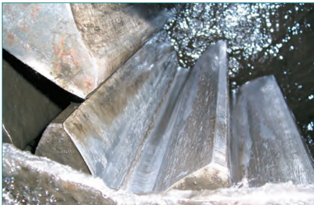
Figure 4. Mild pinion wear and edge plastic flow.
