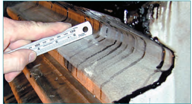
Figure 14. Worn tooth profile with straight edge showing concave shape. (Photo courtesy of The Falk Corp., Milwaukee, WI.)
