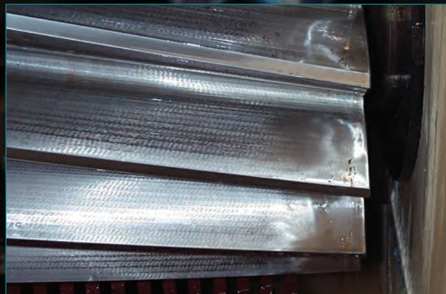
Figure 2. Pinion with original cutting tool marks. Polishing on right side is caused by misalignment.
