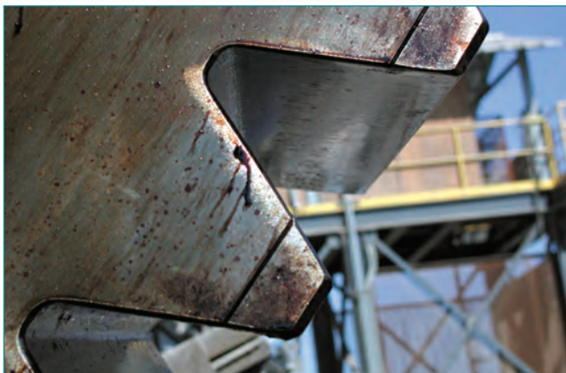
Figure 6. Mild gear profile wear and corrosion.
