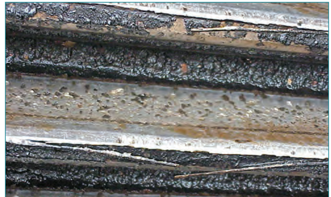
Figure 8. Severe plastic flow results in top land material separation. This material should be removed immediately to prevent debris going through mesh.
