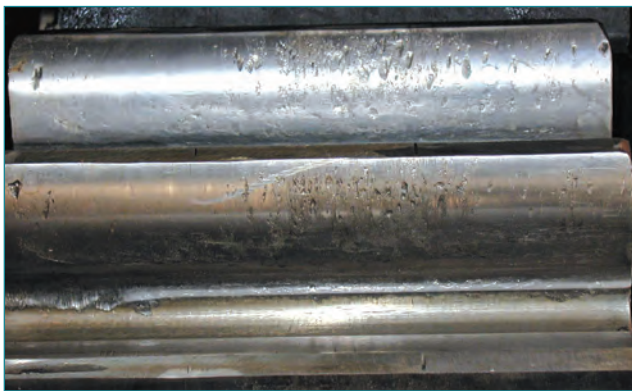
Figure 10. Polishing, debris denting, moderate wear.
