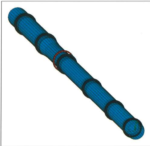
Figure 2. The finite element model for a rotary kiln includes the shell, the riding rings and the ring gear.
